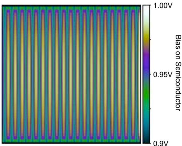
**Figure 6: Spatial bias distribution across a 10cm × 10cm simulated GaAs solar cell**
