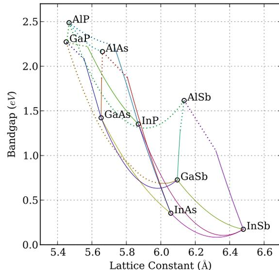
Figure 2: Vurgaftman ternaries parameterisation – dashed lines indicate indirect band gaps
