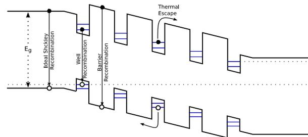
Figure 1: Quantum Well Solar Cell band structure
