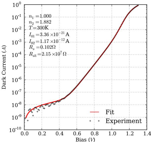
Figure 3: Experimental IV data and fit
