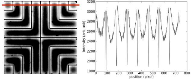
Figure 4: Spatial electroluminescence inhomogeneity due to low front metallisation
