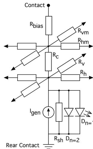
Figure 5: Spatial Grid Equivalent circuit
