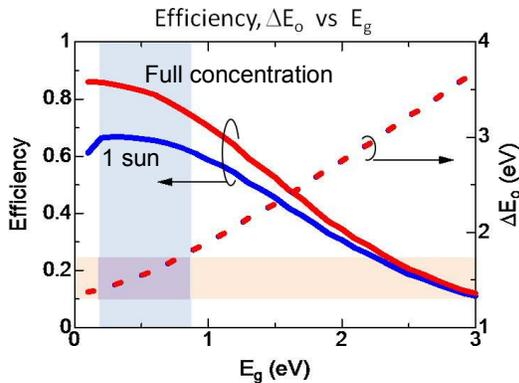
Figure 5 Detailed balance model calculation of the conversion efficiency and required  $\Delta E_o$  vs bandgap energy of absorber.
