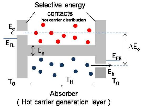
Figure 1 Schematic band structure of a hot carrier solar cell.
