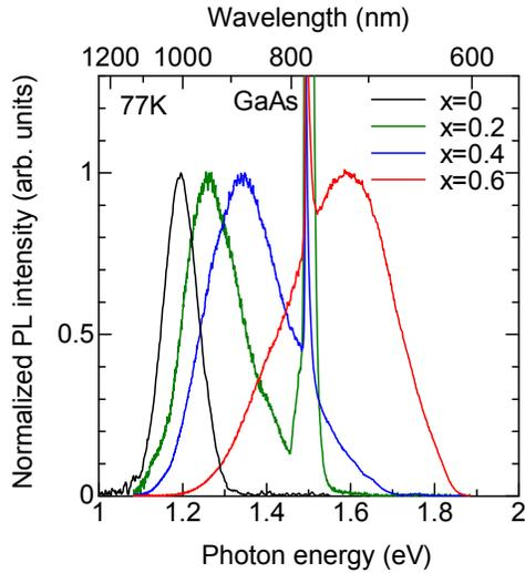
Figure 4 PL spectra of InAs QDs embedded in  $\text{Al}_x\text{Ga}_{1-x}\text{As}$  barrier layers. The intense luminescent peaks at 1.50 eV are from GaAs substrates.
