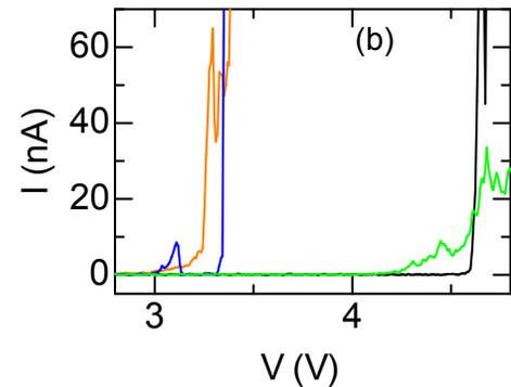
Figure 6 I-V characteristics of InAs QDs embedded in  $\text{Al}_{0.6}\text{Ga}_{0.4}\text{As}$  barriers measured by C-AFM. (a) reverse bias and (b) forward bias. Bias voltage was applied from the substrate to the AFM tip. Current is shown as absolute value in the figures. Each curve indicates a measurement result at different positions on the sample surface.
