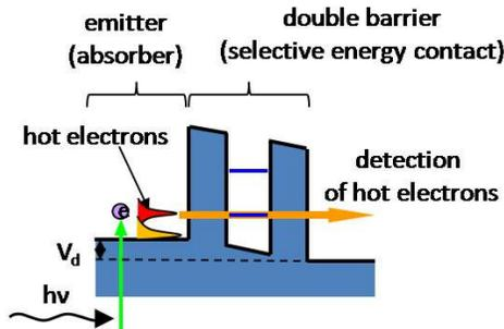
**Figure 2** A schematic illustration of photo-generation of hot carrier distribution and its extraction through a DB resonant tunneling structure.
