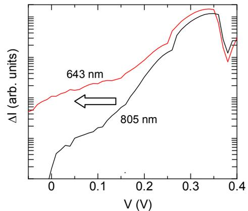
**Figure 3** Dependence of the current increase induced by light excitation on applied voltage. The excitation wavelengths are 643 nm (red line) and 805 nm (black line).
